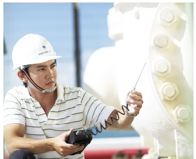
Routine checks for gas leakage ensure safety
