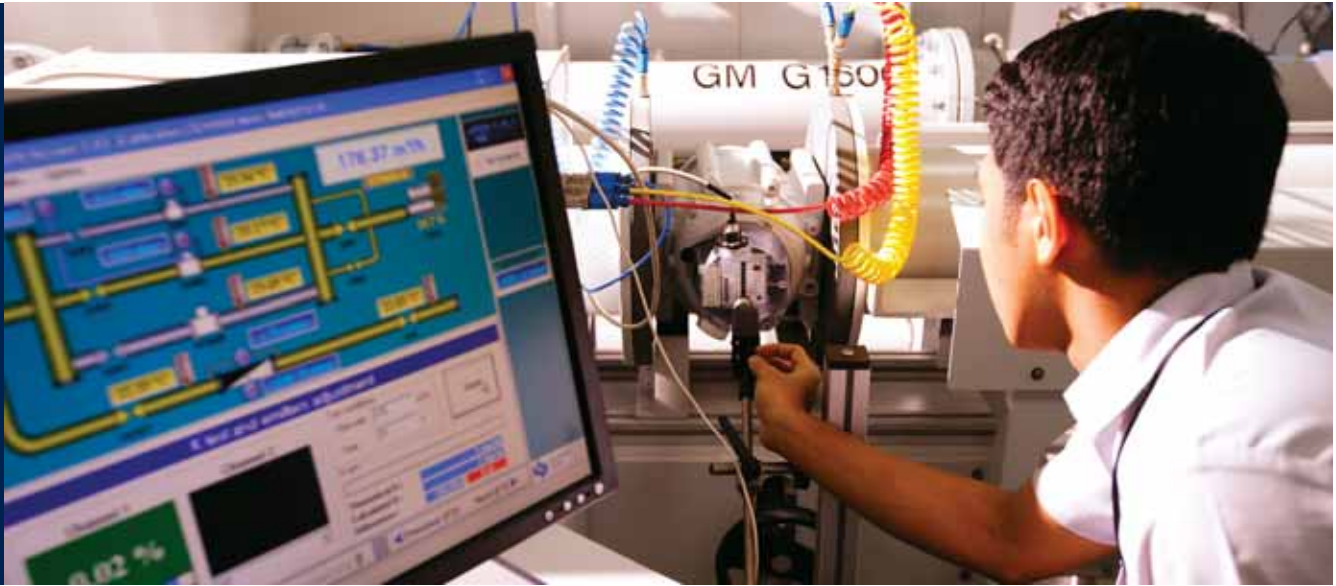
Calibrating gas meters at the Meter Laboratory
