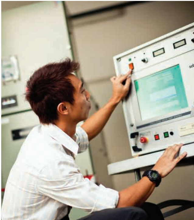
Cutting-edge Oscillating Wave Test equipment helps engineers monitor the condition of high voltage cables.
