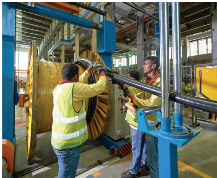
The Automated Coiling Machine supports our productivity process by reducing the manpower required and time taken to re-coil cables.
